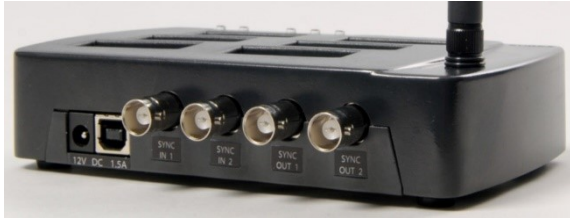
Figure 2 - Awinda Station. 4 BNC ports: SYNC IN 1, SYNC IN 2, SYNC OUT 1, SYNC OUT 2.
