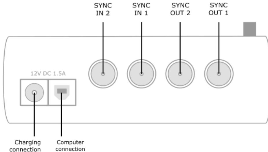
The Xsens Awinda and Sync Stations have four BNC connectors, with two Sync IN and two Sync OUT possibilities. These hardware connections are shown in Figure 1.
