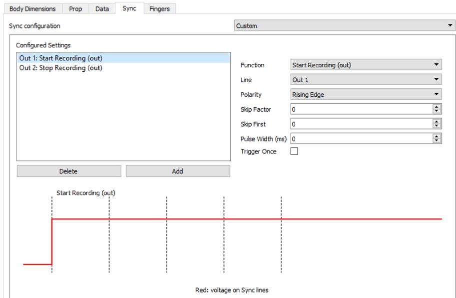
Figure 5 - Motion Capture Configuration window in MVN Analyze. Setting on the sync tab.
