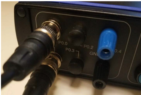
Figure 4 - Connection with BNC-BNC cable scheme to Start and Stop a recording.
