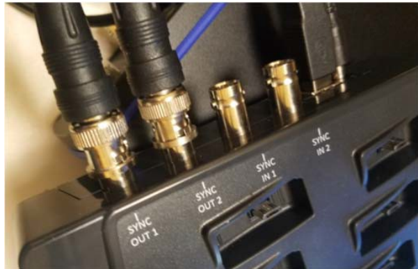
Figure 4 - Connection with BNC-BNC cable scheme to Start and Stop a recording.
