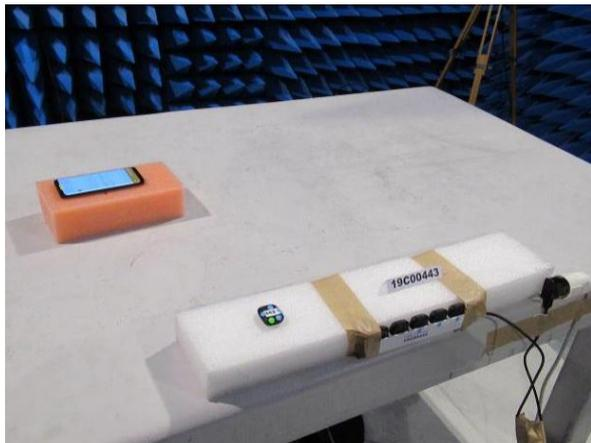
Picture 3: Radiated emission test setup
