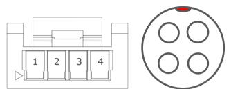
Figure 19: Numbering 4-pin connectors; left Mofex (cable entry view), right ODU (solder cup view).
