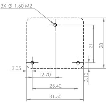
Figure 13: Standalone mounting hole positions (dimensions in mm)
