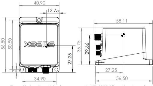
Figure 10: Location origin of measurements MTi-680G (dimensions in mm)
