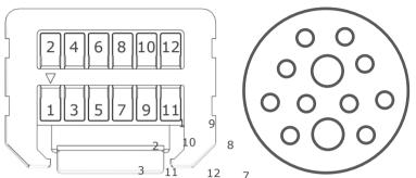
Figure 17: Numbering 12-pin connectors; left Molex (cable entry view), right ODU (solder cup view).6 4
