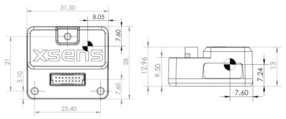
Figure 9: Location origin of measurements module (dimensions in mm)
