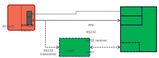
Figure 5: Connections for the GNSS interface
