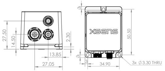
Figure 14: MTi-680G connector and mounting hole positions (dimensions in mm)
