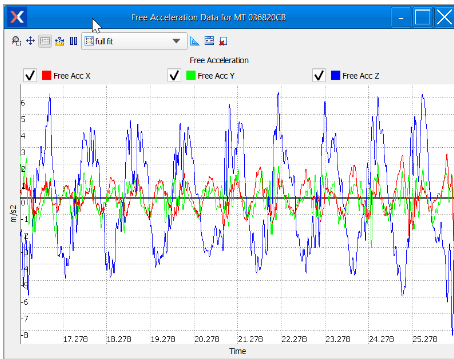
Figure 30: The Free Acceleration view, visualizing 3D Free Acceleration in m/s^2
