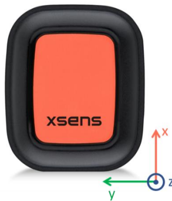
Figure 10: Xsens DOT sensor coordinate system
