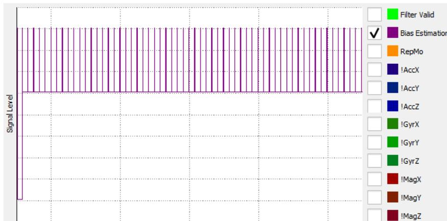
Figure 10: The Status Word output of the MTi-630 showing periodical Manual Gyro Bias Estimation calls. However only the first call (before the robot took off from its docking station) succeeded. All other calls were automatically rejected by the MTi-630 because the device was not motionless.
