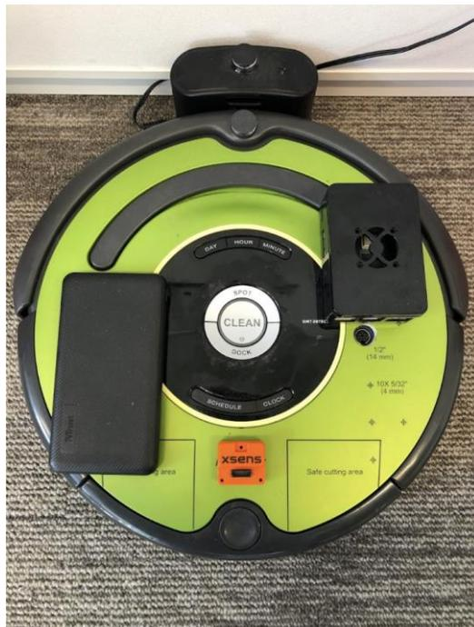
Figure 9: The vacuum robot connected to its docking station. Mounted on top are the encased Raspberry Pi 4B, a power bank and the MTi-630. All connections (not shown on the photo) were established through USB.
