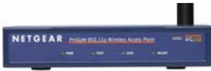
Figure 9: Netgear ProSafe 802.11G Wireless Access Point.
