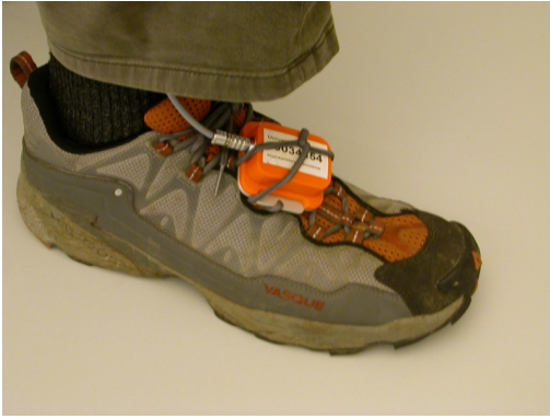
Fig. 1. An Xsens MT motion sensor is held on to the shoe by the laces. In principle, the IMU could be miniaturized and mounted in the heel or insole of a boot.
