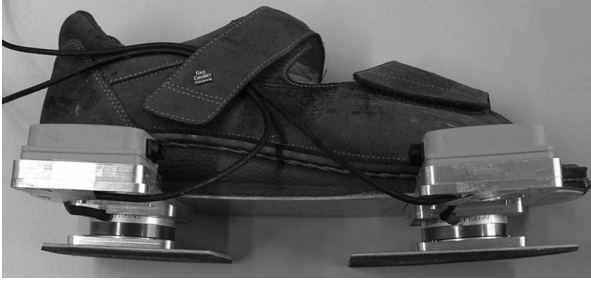
Fig. 1. Picture of the instrumented shoe with force/moment sensors beneath the heel and forefoot and inertial sensors rigidly attached to the force/moment sensors.
