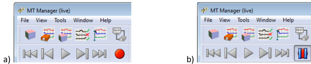
Figure 8: Record button in MT Manager. a) before clicking b) after clicking, with sync-in activated.
