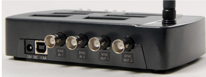
Figure 1: Xsens Awinda Station showing the four BNC connections for synchronisation purposes
