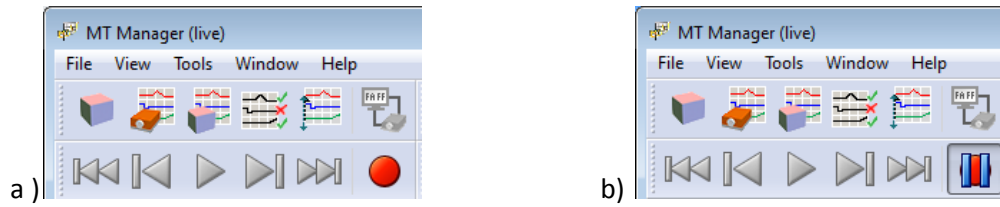
Figure 4: Record button in MT Manager. a) before clicking b) after clicking, with sync-in activated.
