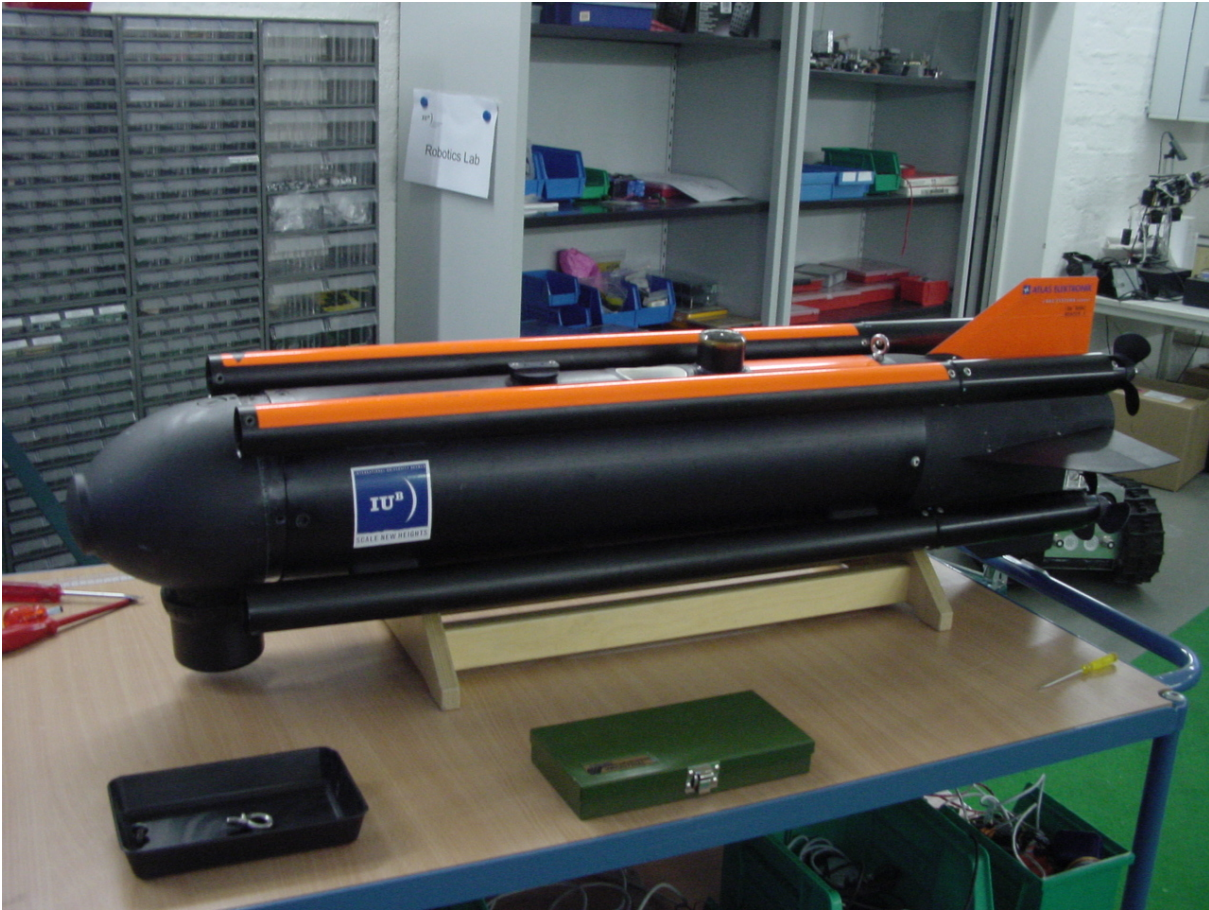
Figure 4: Some of the most basic vehicle parts, namely the hull, the motors and the batteries, are based on parts from a so-called Seafox ROV that was provided by ATLAS ELEKTRONIK to IUB. The complete development of the electronics, the sensors, the onboard computer, the actuators, and software was solely done by the IUB team.
