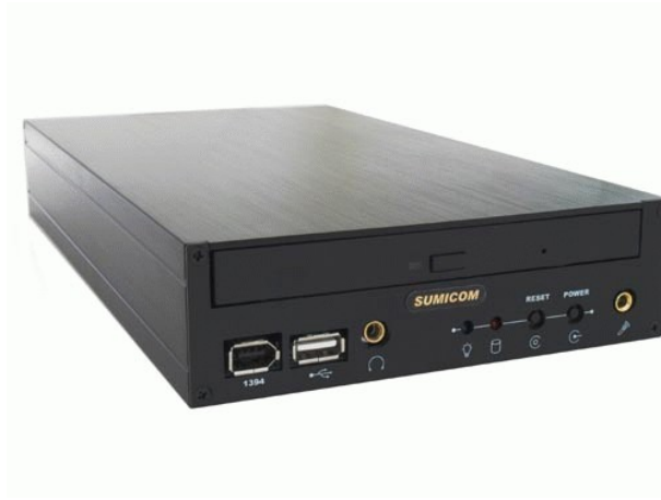
Figure 10: The Sumicom S625F as “cognition” unit on the IUB AUV.
