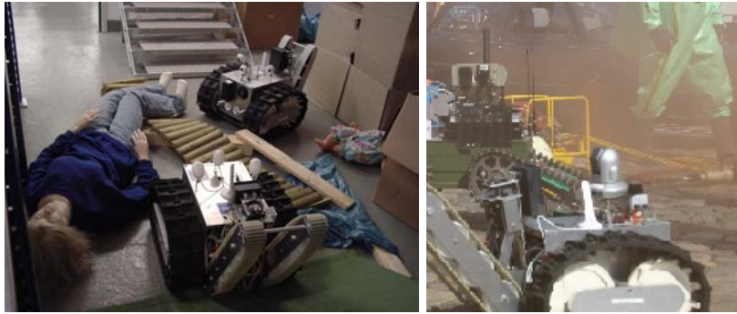
Figure 2: Two IUB rescue robots in a test arena in the robotics lab (left) and an IUB robot participating in a disaster drill involving hazardous materials (right).
