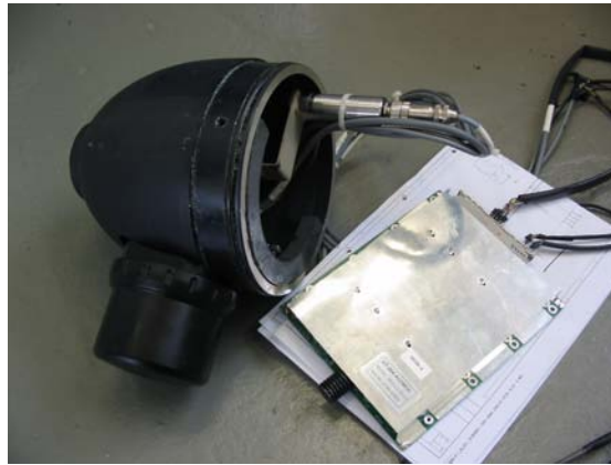
Figure 11: The nose of the submarine with the seeking sonar (the black cylinder underneath). The sonar board and the cables leading to it are also visible. The metal stick coming out of the top of the nose is the pressure sensor.
